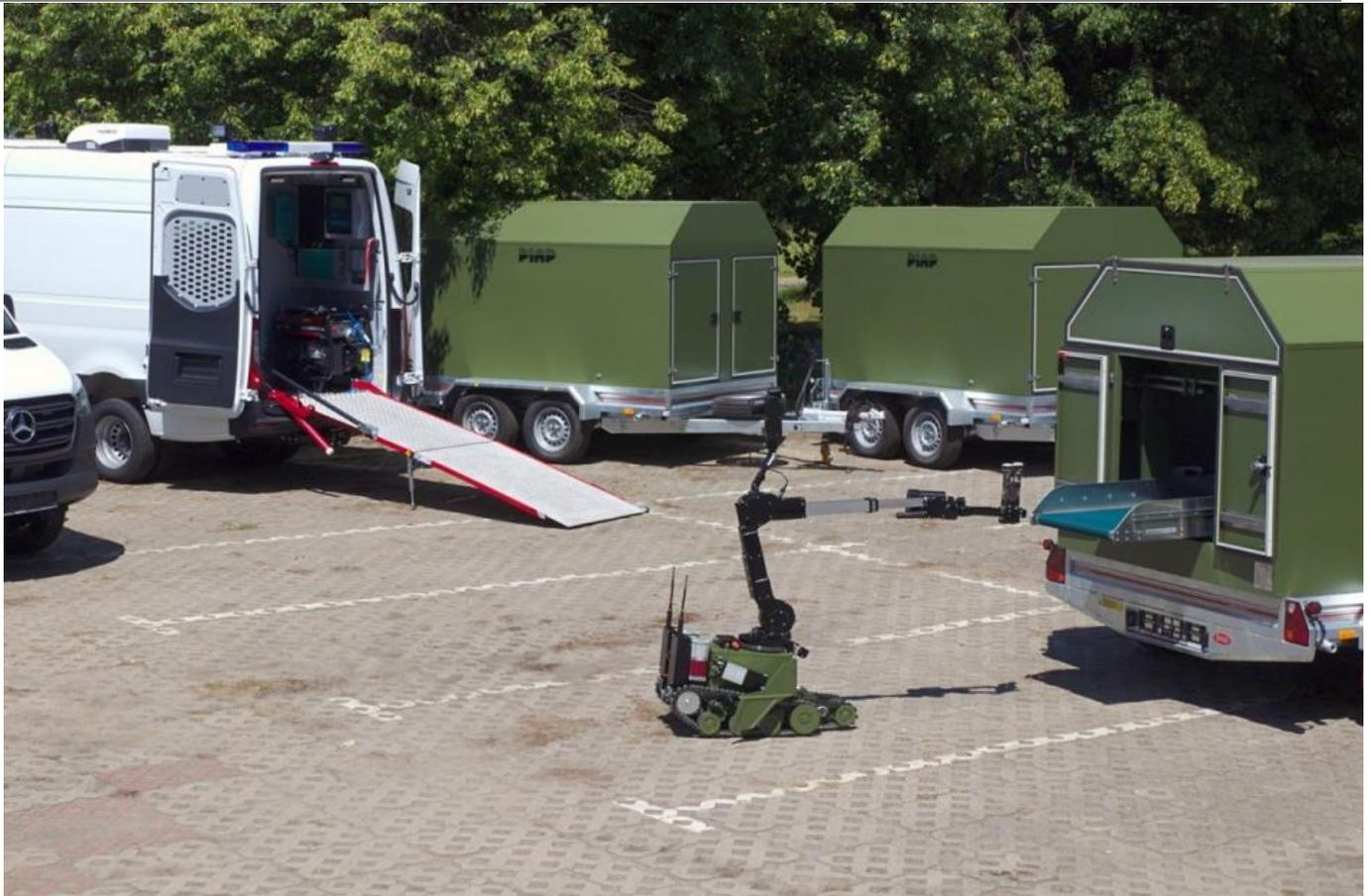
*The Vietnamese Army, which will be the main operator of PIAP's pyrotechnic sets, had already worked out a special tactic for dealing with EOD-like threats. However, the service lacked proper equipment. The systems, which were delivered by Lukasiewicz – PIAP Institute, will be used mainly to conduct reconnaissance and neutralization of improvised explosive devices (IED) and other potentially hazardous materials / Picture: Lukasiewicz – PIAP Institute*
