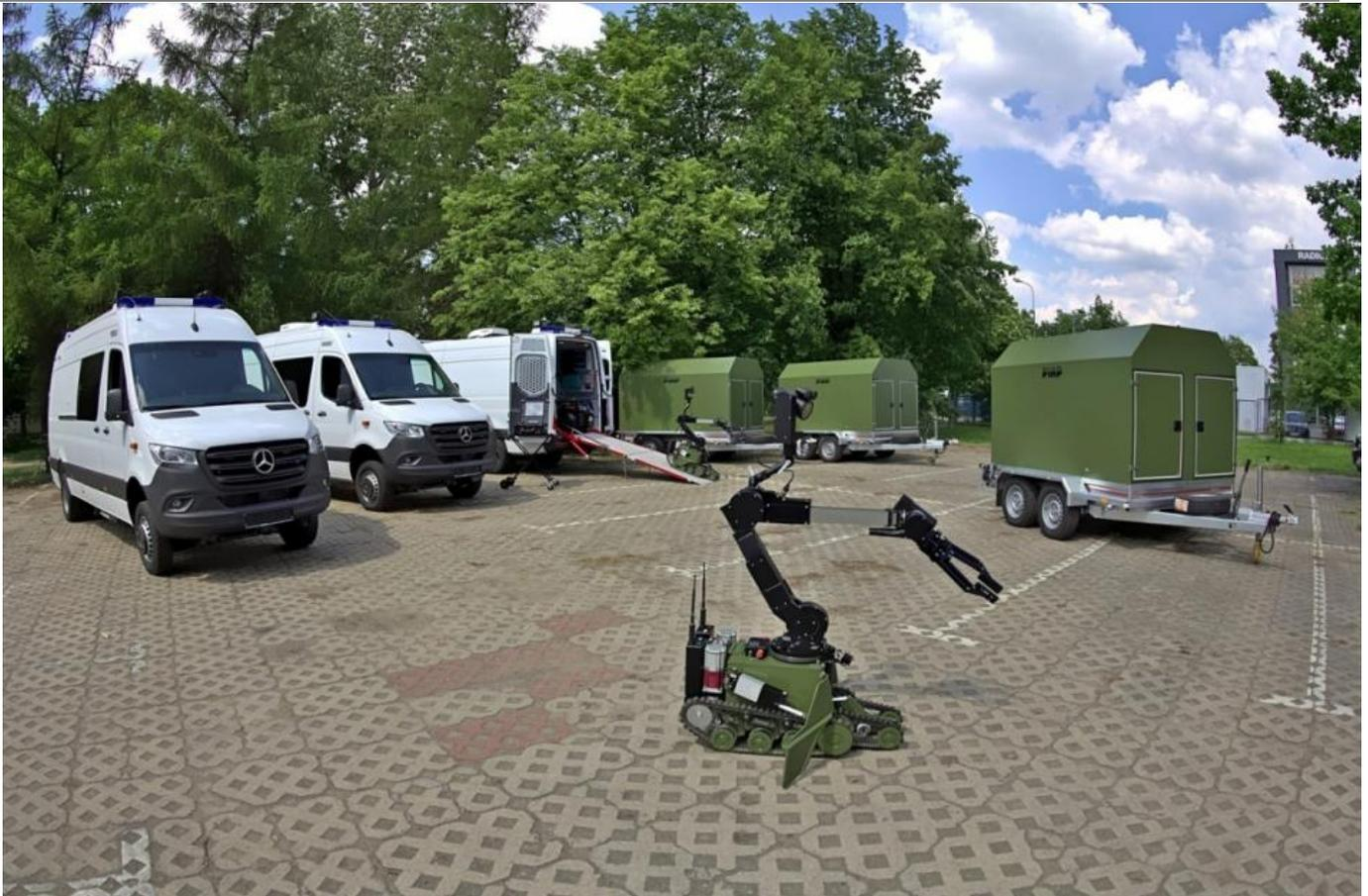
*The Lukaszewicz - PIAP Institute delivered counter-EOD sets to Vietnam. Each one of them consisted of a pyrotechnic ambulance based on the Mercedes Sprinter vehicle, along with auxiliary equipment, an EOD robot and a trailer with a Vera-type based ventilated explosion containment vessel with resistance to explosion of up to 5kg in TNT equivalent from our Jakusz partner / Picture: The Lukaszewicz - PIAP Institute*
