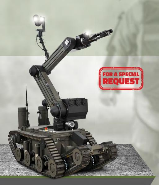
Track drive system with articulated front flippers enhances traction and allows to work both in difficult terrain and inside buildings, where it performs activities such as climbing stairs regardless of lighting and atmospheric conditions (within the limits defined by technical parameters of the device).
