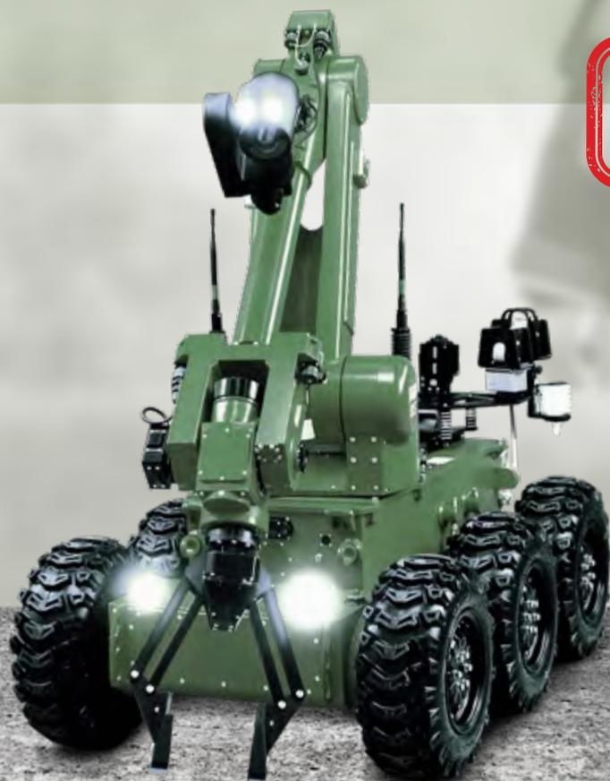
PIAP IBIS® is a fast robot (10 km/h). Special design of mobile base suspension ensures optimum wheel contact with the ground. Precision drive system ensures fluidity of the movement of every part of the robot, at any speed.
