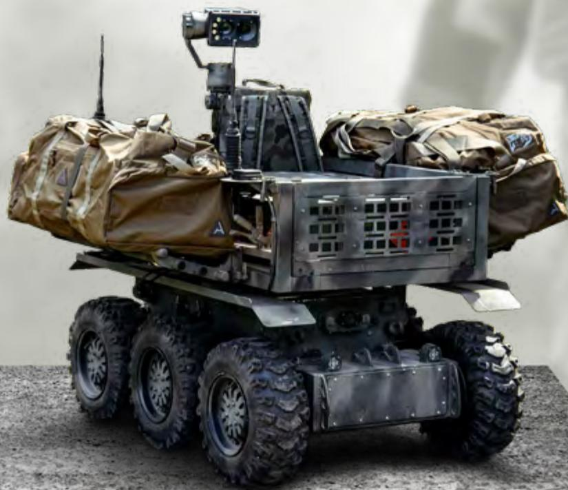
The PIAP IBIS robot can be controlled from the PIAP HUNTeR robot control panel and can serve as observation support thanks to the installed PTZ head with a day-night camera with zoom and a thermal imaging camera. Radio control of a smaller robot in a network with a PIAP HUNTeR combat robot allows for mutual transmission of a radio signal, extending the operational range of one or the other unmanned platform.
