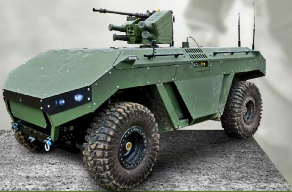
The vehicle is equipped with a 3-link dependent suspension with a Panhard rod coil springs and shock absorbers with controlled damping. Łukasiewicz-PIAP used a differential lock and two steering axles.
